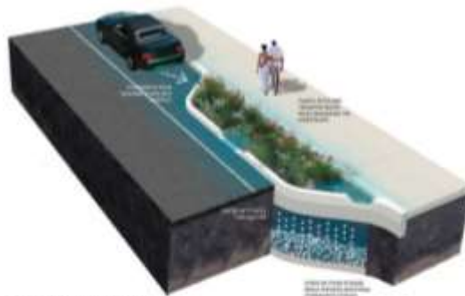
Mid-block Stormwater Bump-out
